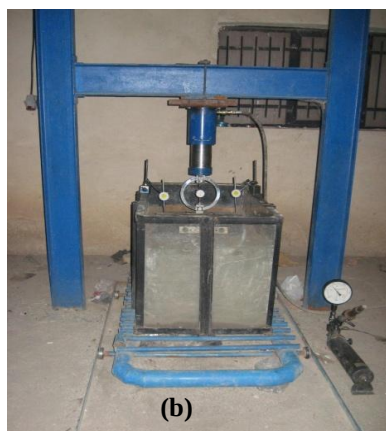
Figure 5. Vibratory tamper and test box during loading
